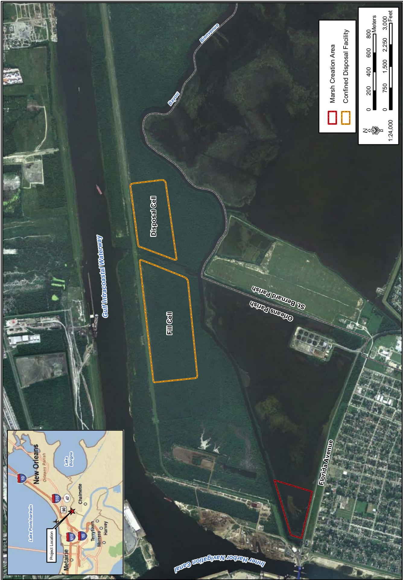
Figure 4-10: Float-in-Place Confined Disposal Facility Option #2
